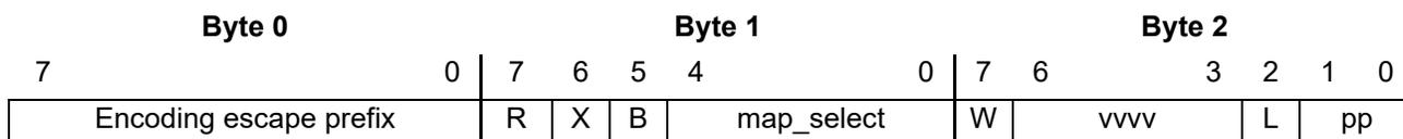
Figure 1-7. VEX/XOP Three-byte Escape Sequence Format
